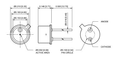
Note: Lead soldering temperature (1/16 inches from case) 260°C for 3 sec.
