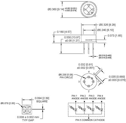
> Soldering Conditions: 260°C 1/16 inch away from case for 3 seconds max.
