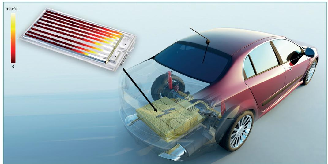
The Luna Optical Distributed Sensor Interrogator (ODiSI) (below) is an advanced strain and temperature measurement system helping engineers to overcome energy storage system design challenges for electric and hybrid automotive applications (above)
