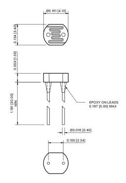
Note: Lead soldering temperature (1/16 inches away from body) 260°C for 3 sec.
