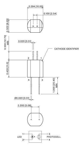
Note: Lead soldering temperature (2mm away from case) 260°C for 5 sec.
